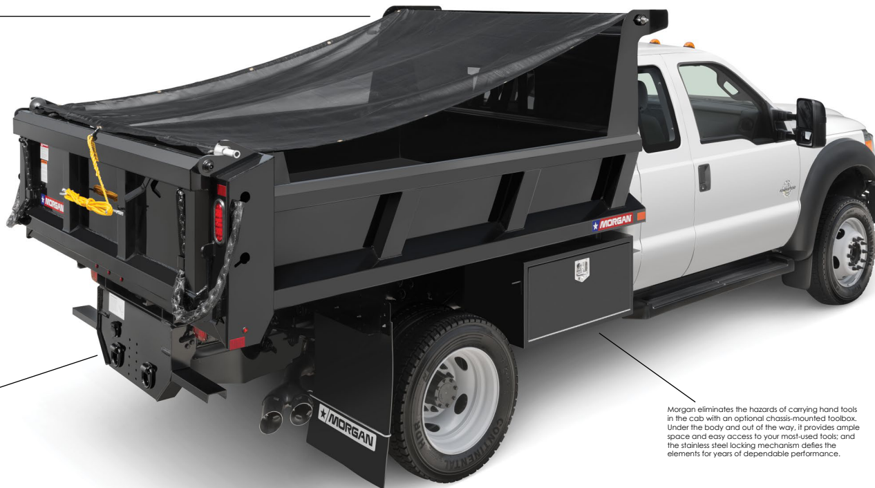
Morgan's heavy-duty hitch plate and tow rings make it easy to mount any hitch configuration and safely tow. The plate-mounted plug-n-play light connector also supports quick, easy and dependable trailer light hook-up. The use of OEM lighting modules also supports easy repair and replacement if needed.
