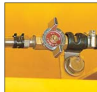
Fuel Drain Valve
