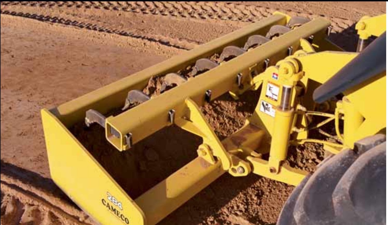
84-inch Cameco box scraper employs a high-volume back, double-beveled reversible cutting edge, and high-lift scarifier with heat-treated replaceable teeth.
